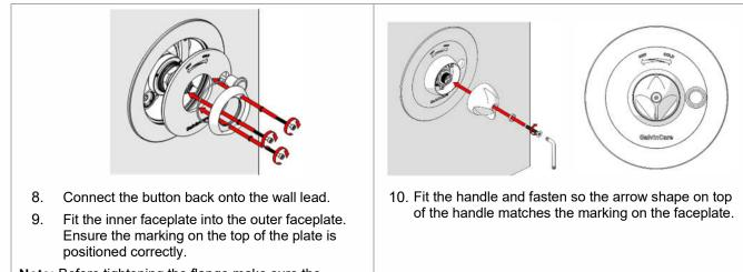
**Note:** Before tightening the flange make sure the handle fits correctly. Put screws into flange and tighten finger tight, the flange should still be able to move. Slide the handle onto spline and move the flange until central to the handle. Remove handle and tighten the screws (it is best to tighten the screws in sequence a little at a time to avoid the flange moving). Refit handle.
